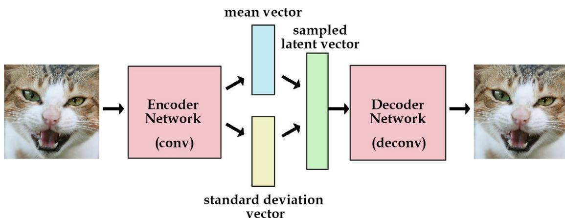
Figure 1: Basic structure of a variational autoencoder [8]
